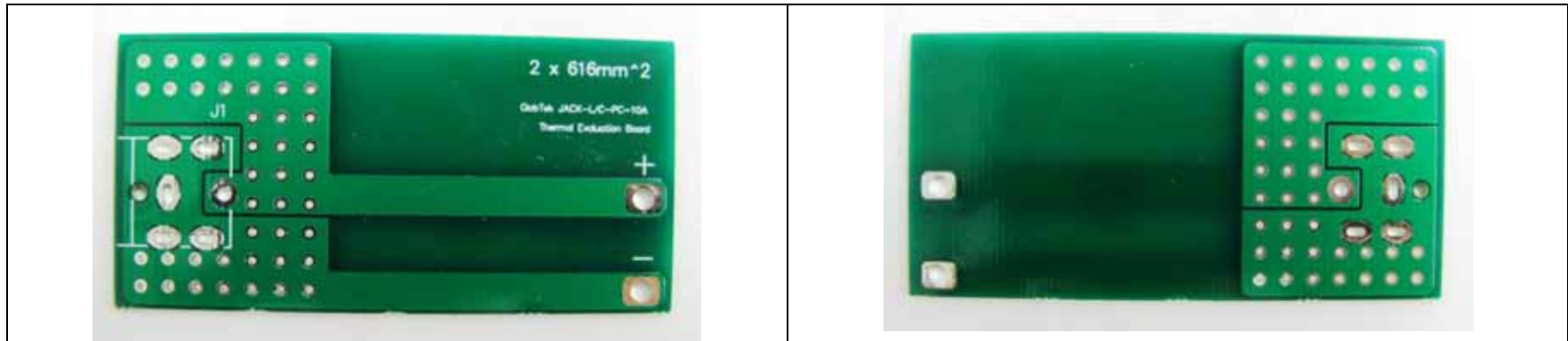
GLOBTEK RECOMMENDED MOUNTING BOARD FOR THE CONNECTORS
